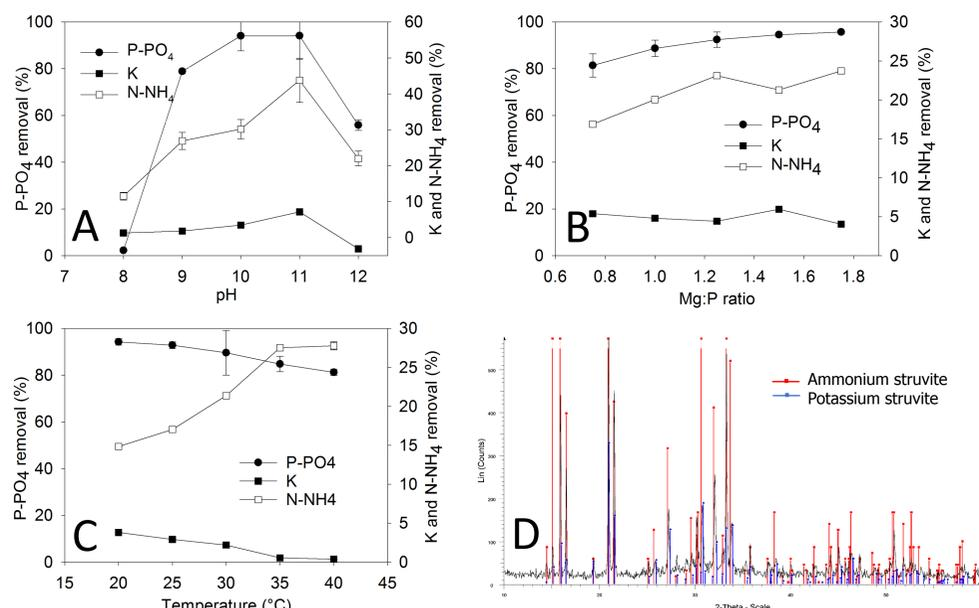
Figure 2 – Influence of pH (a), Mg:P ratio (b) and temperature (c) on nutrient removal, and a diffractogram obtained from precipitates at pH 11, Mg:P ratio 1.25 and 25°C
